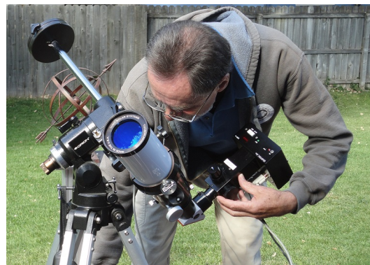
Figure 1: (left) A month of H and J band data collected with the SSP-4 photometer from Optec. (right) Myself lining up the Lunt 60 mm tilt-etalon solar scope with the SSP-4 photometer at the eyepiece.
