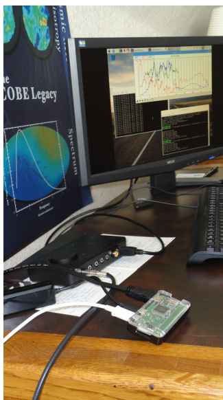
Figure 1: The Xonar external sound card (black box) and Pi Zero computer (foreground)
