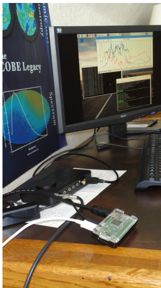
Figure 4: The Xonar external sound card (black box) and Pi Zero computer (foreground)
