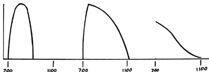
Figure 1. Low-budget sketch of (l-r) Cousins I, RG9, and CCD (KAF-16803) response curves.
