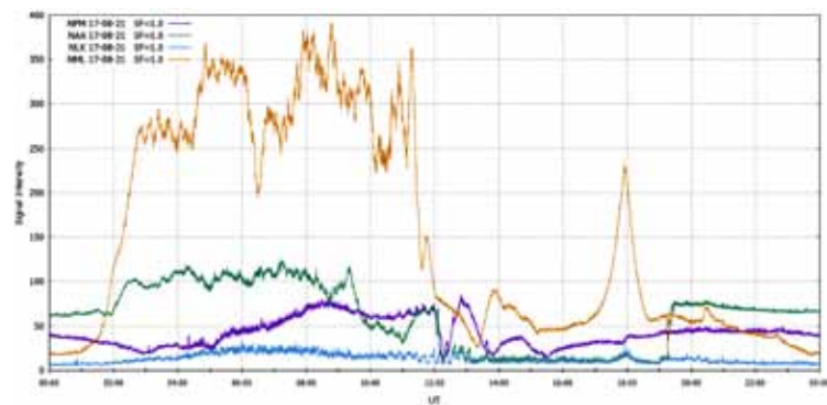
Figure 3. All Naval transmitters and their response to the eclipse from Ft. Collins, Colorado.
