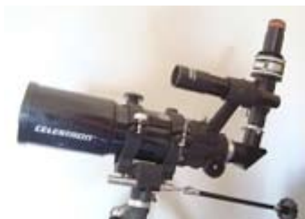
80-mm f/5 refractor for H-alpha solar observations
