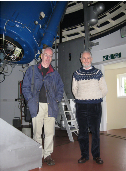
John and Tom with the Gregory telescope. This 0.94-m (37-inch) Schmidt-Cassegrain reflector is fitted with a research quality CCD camera for direct imaging and has the distinction of being the largest operational optical telescope in the UK.
