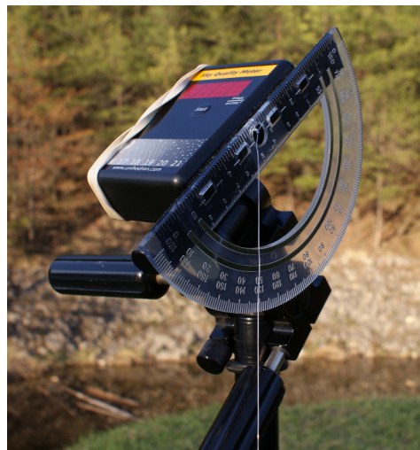
Figure 1b. To measure zenith angles, we attached a simple protractor with plumb-line to the side of the SQM using adhesive Velcro tape.
