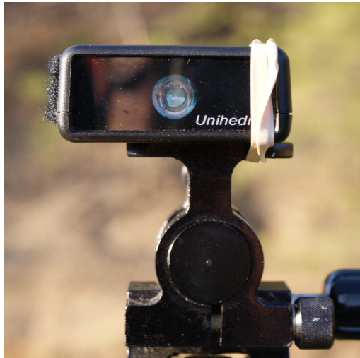
Figure 1a. Mounting the SQM-L on the tripod shoe pad can be done quite simply and quickly with the use of a thick rubber band.
