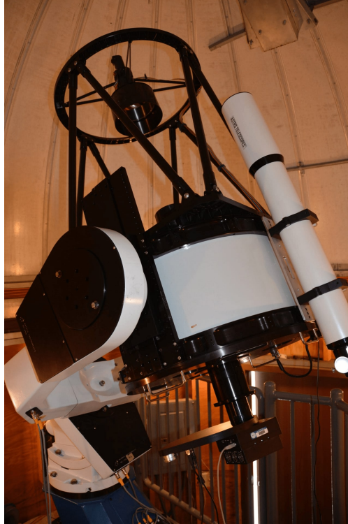
Figure 3. The 0.51-meter f/8 Ritchey-Chrétien reflecting telescope at WMO.
