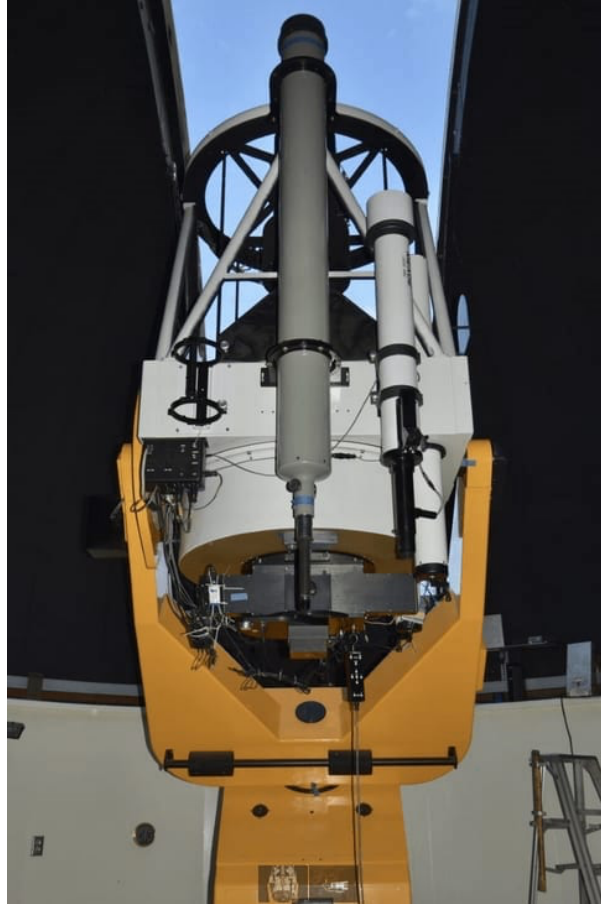
Figure 2. The 0.91-meter f/5.5 Ritchey-Chrétien reflecting telescope at WMO.
