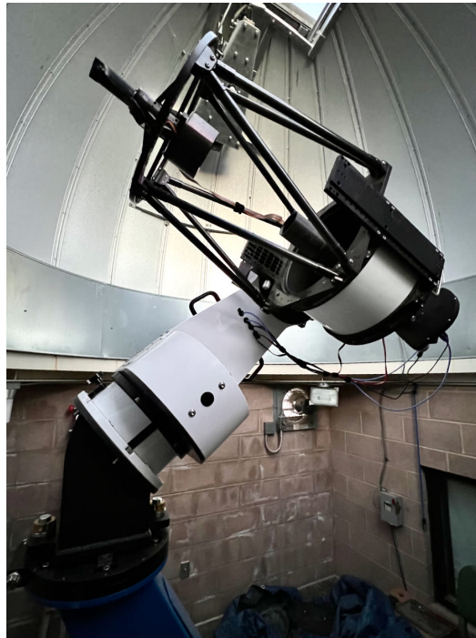
Figure 4. The 0.32-meter f/9 Ritchey-Chrétien reflecting telescope at WMO.
