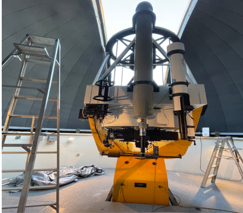
Figure 2. The 0.91-meter telescope, the main reflector telescope used to observe the candidates for this project.
