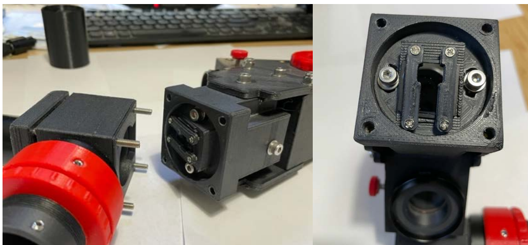
Figure 5. Disassembly of the slit holding compartment of the StarEx; on the right, a close-up or the small parts holding the slit in place (no slit is present in this photo).
