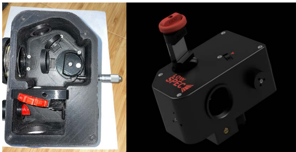
Figure 3. Interior of the LowSpec, and an illustration from the assembly manual (Gerlach 2021) showing how the grating is removed and replaced.
