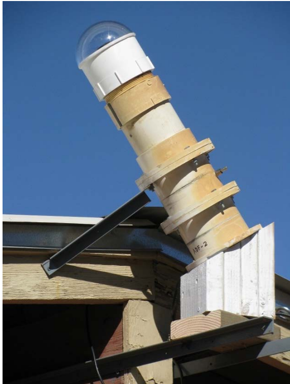
Fig. 1. Sandia video camera housing. System incorporates PVC fittings for waterproofing with internal heater and power supply.
