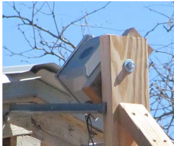
Fig. 2 Second generation camera housing with 100 degree field of view.
