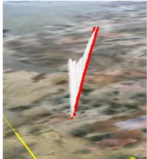
Fig. 7 White vertical lines above the red reentry path indicated the relative brightness during the burn phase. In this configuration the light curve can be visually correlated to the penetration into the atmosphere.
