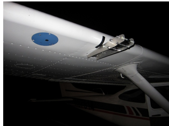
Figure 4. LANM Model 5 and LANM Model 6 mounted on a C-182Q aircraft wing. The former is on the cantilevered mount, and the latter inside the blue wing panel.
