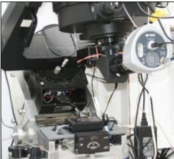
Figure 13. The Orion Observatory's Andor Luca-S camera and 10-inch telescope equipped with a Sidereal Technology control system.
