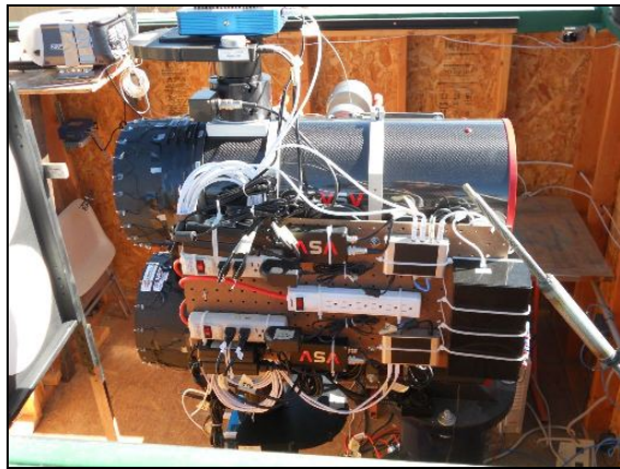
Figure 2. The twin 8-inch APASS-North astrographs at Tom Smith's Dark Ridge Observatory in Weed, New Mexico.
